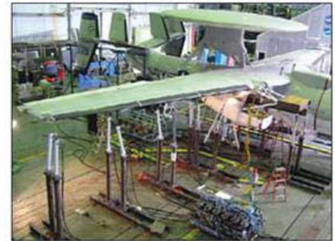
Conventional Loads Calibration Setup
