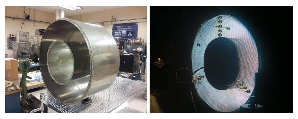
Images of GEN2 (65 cm dia.) Annular Engine hardware, from left-to-right: annular discharge chamber, sans magnetics, undergoing assembly; annular discharge chamber in vacuum undergoing simulated beam extraction tests, with high-transparency grid-plate and embedded probes on downstream end of discharge chamber.
