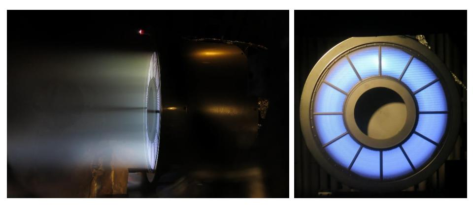
Images of 65 cm dia. Annular Engine beam extraction tests, left-to-right: side-view showing beam propagation; head-on view of engine. Neutralizer cathode assembly is at 12-o'clock position (left image) and is cropped (right image) due to beam target surface in camera field-of-view.
