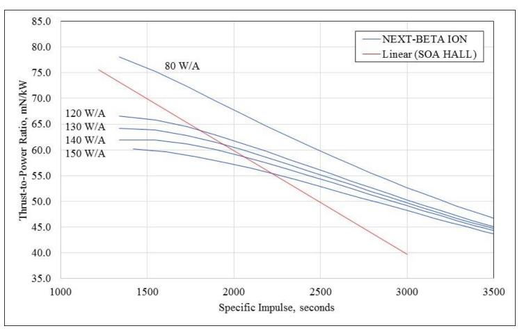
With minor magnetic circuit modifications and higher current density, lower discharge losses should be readily obtainable; at least to 150 W/A. At 150 W/A, the cross-over point where  $F/P_{in}$  for ion engines exceeds that for HETs is reduced from 2,600 seconds (for SOA engines) to about 2,300 seconds  $I_{sp}$  – with further improvements in  $\varepsilon_i$  lowering the cross-over further
