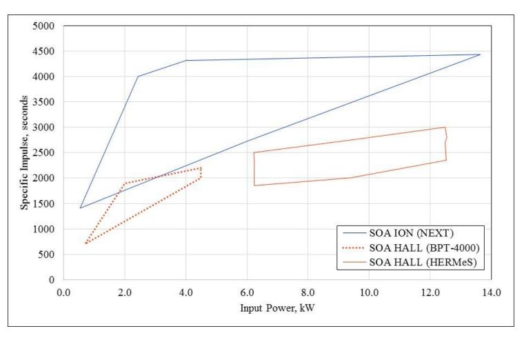
While NEXT has a larger demonstrated throttling range in both specific impulse and input power, it does so for the most part at a lower  $F/P_{in}$  parameter
