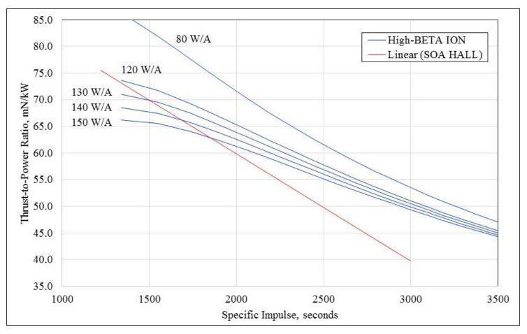
In this instance, minor improvements in magnetic circuit design in combination with flat ion optics should drive the cross-over point where the  $F/P_{in}$  parameter for ion engines exceeds that for HETs from 2,600 seconds down to about 1,800 seconds  $I_{sp}$
