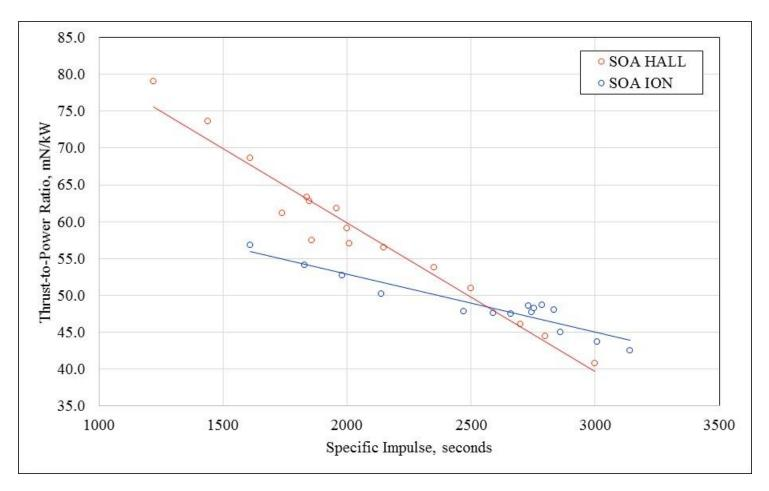
Curve fits of both the SOA HALL and SOA ION data indicate a cross-over in  $F/P_{in}$  at about 2,600 seconds lsp, with HETs having superior  $F/P_{in}$  below 2,600 seconds, and ion engines having superior  $F/P_{in}$  above 2,600 seconds – including at the intended HERMeS operating condition of 3,000 seconds
