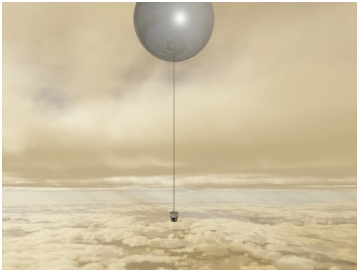
Figure 5.—Venus Super-Pressure Balloon Concept Illustration (Ref. 5).
