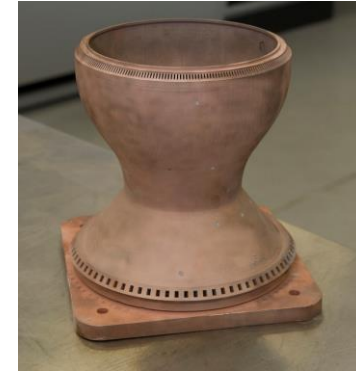
GRCop-84 Liners produced by SLM
