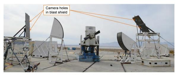
Figure 18.—High-speed camera locations for digital image correlation; four cameras, two per panel.
