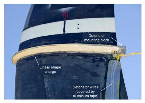
Figure 27.—Linear shape charge final installation.
