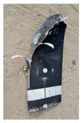
Figure 40.—Upper blade after impact on 24-ply composite panel.
