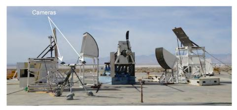
Figure 23.—Cameras used to measure blade kinematics.
