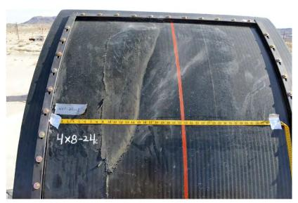
Figure 36.—24-ply composite panel postimpact damage, front side.
