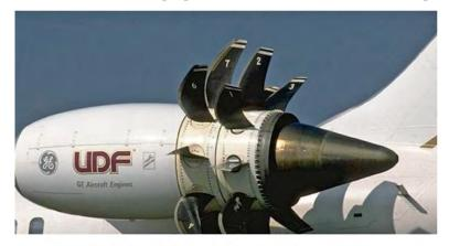
Figure 1.—General Electric (GE) unducted fan demonstrator.
