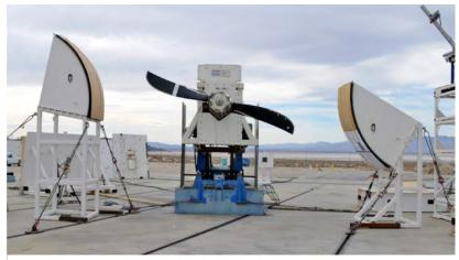
Figure 6.—Spin rig on T406 spin fixture.
