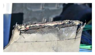
Figure 10.—Blade section at cut line.
