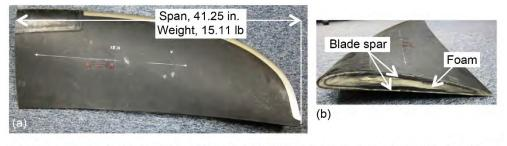
Figure 5.—Candidate blade configuration for shield impact. (a) Outer blade length and weight. (b) Blade cross section.
