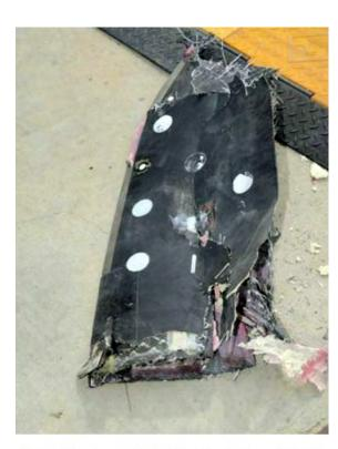
Figure 34.—Lower blade after penetration of 20-ply composite panel.
