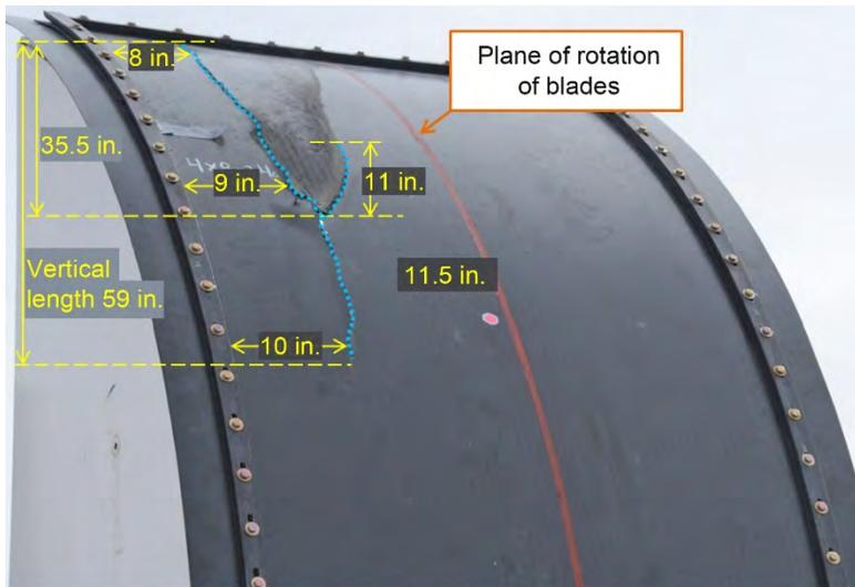
Figure 38.—24-ply composite panel, front side, with measurements.
