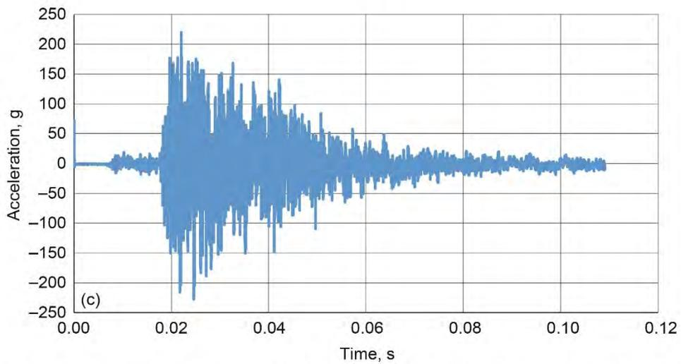
Figure 60.—Accelerometer response for 24-ply panel. (a) P24–X1. (b) P24–Y1. (c) P24–Z1.
