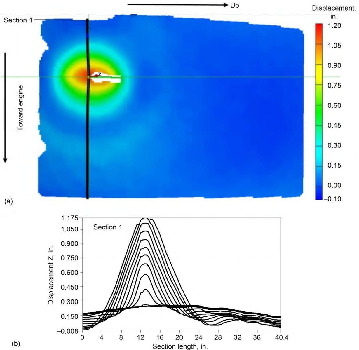
Figure 43.—Inward radial displacement of 20-ply panel after blade penetration. (a) Contour plot just prior to failure. (b) As function of length along segment line shown in part (a) for several frames up to time of maximum deflection; time between each line is 66.7 ms.
