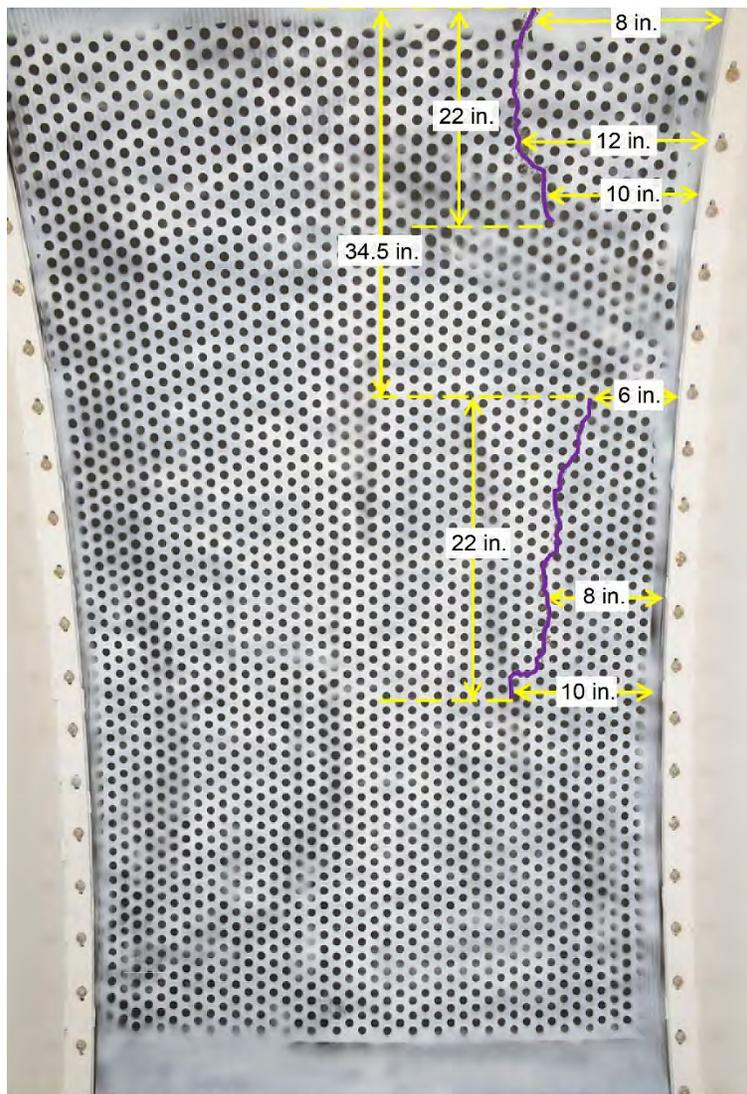
Figure 39.—24-ply composite panel, back side, with measurements.
