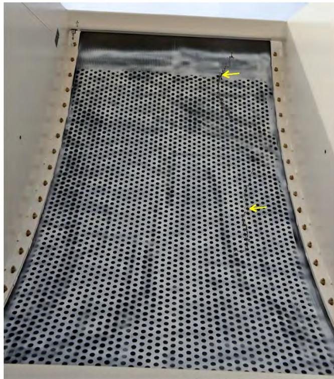
Figure 37.—24-ply composite panel postimpact damage, back side.
