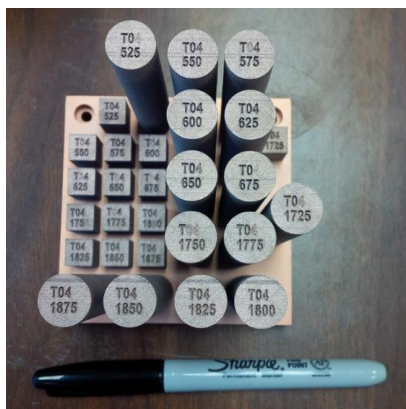
Fig. 8: Example of GRCop-84 samples used for analysis.
