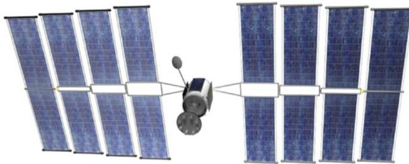
Figure 3. HEFT 300-kW SEP Vehicle Concept [2011].
