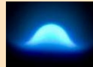
Coflow Laminar Diffusion Flame (CLD Flame)
