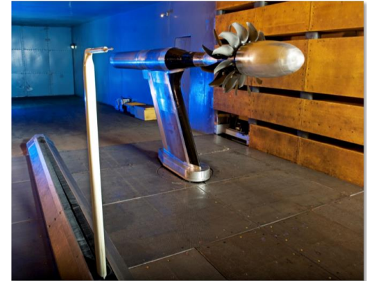
Fan and CROR rigs in NASA GRC 9- by 15-ft low speed wind tunnel
