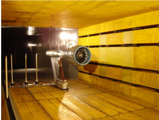
Fan and CROR rigs in NASA GRC 9- by 15-ft low speed wind tunnel
