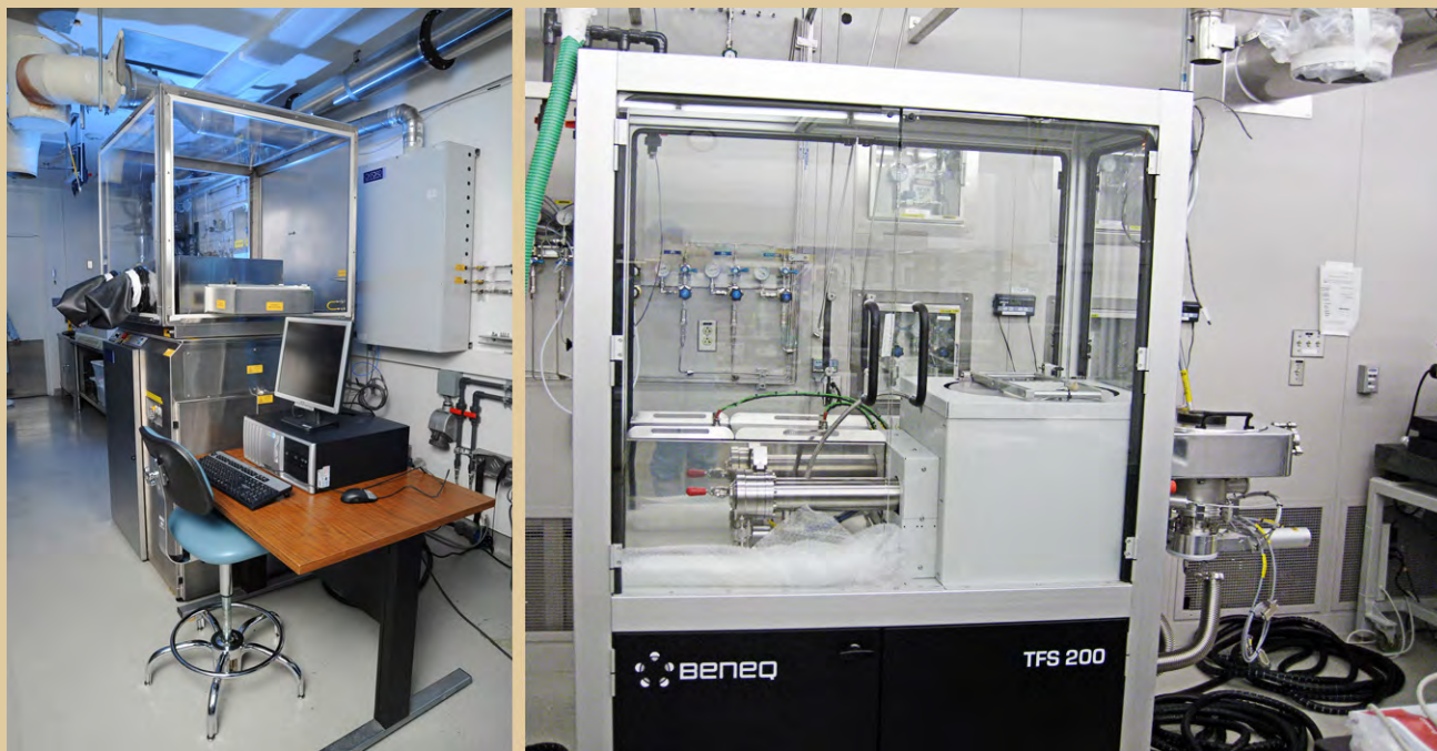
Fig. 5. JPL ALD systems. Both systems can accept samples/wafers up to eight inches in diameter. Most work is done at die level in order to maximize the number of runs on a single die (there are 17 dice of this format on a six-inch wafer).
