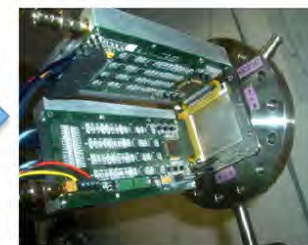
Two small, low-mass, low-power ASIC and FPGA boards qualified for flight
