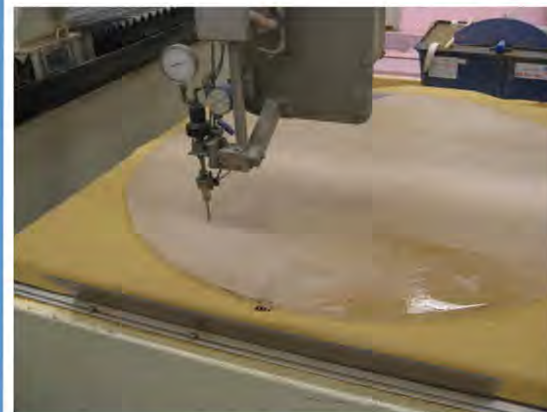
Rounding the glass face plate
