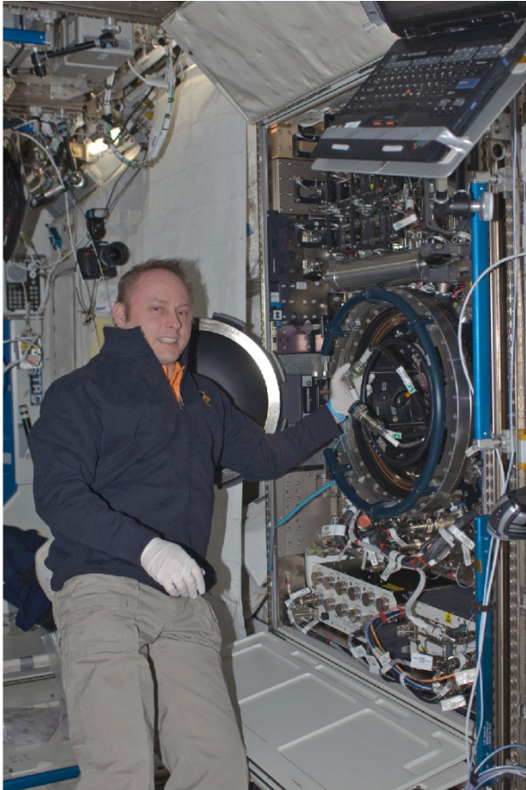
Figure 1.—Astronaut Mike Fincke to the left of the Combustion Integrated Rack (CIR) facility shortly after it was installed in the Destiny module of the International Space Station (ISS).
