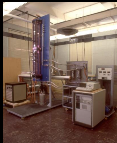
Falling-Film Heating/Evaporation Facility
