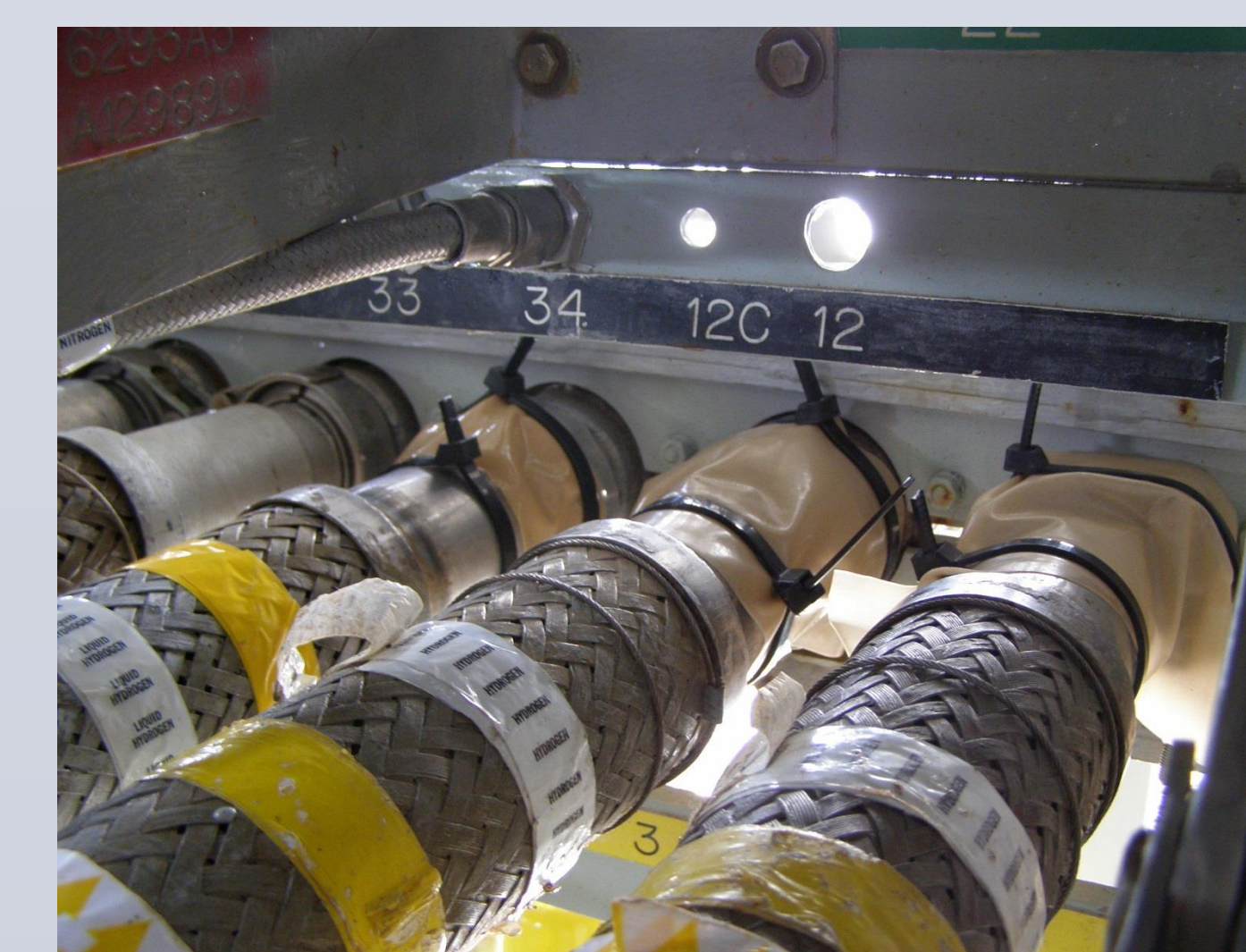
Deployment of tape on hydrogen fuel cell lines during STS-120.
