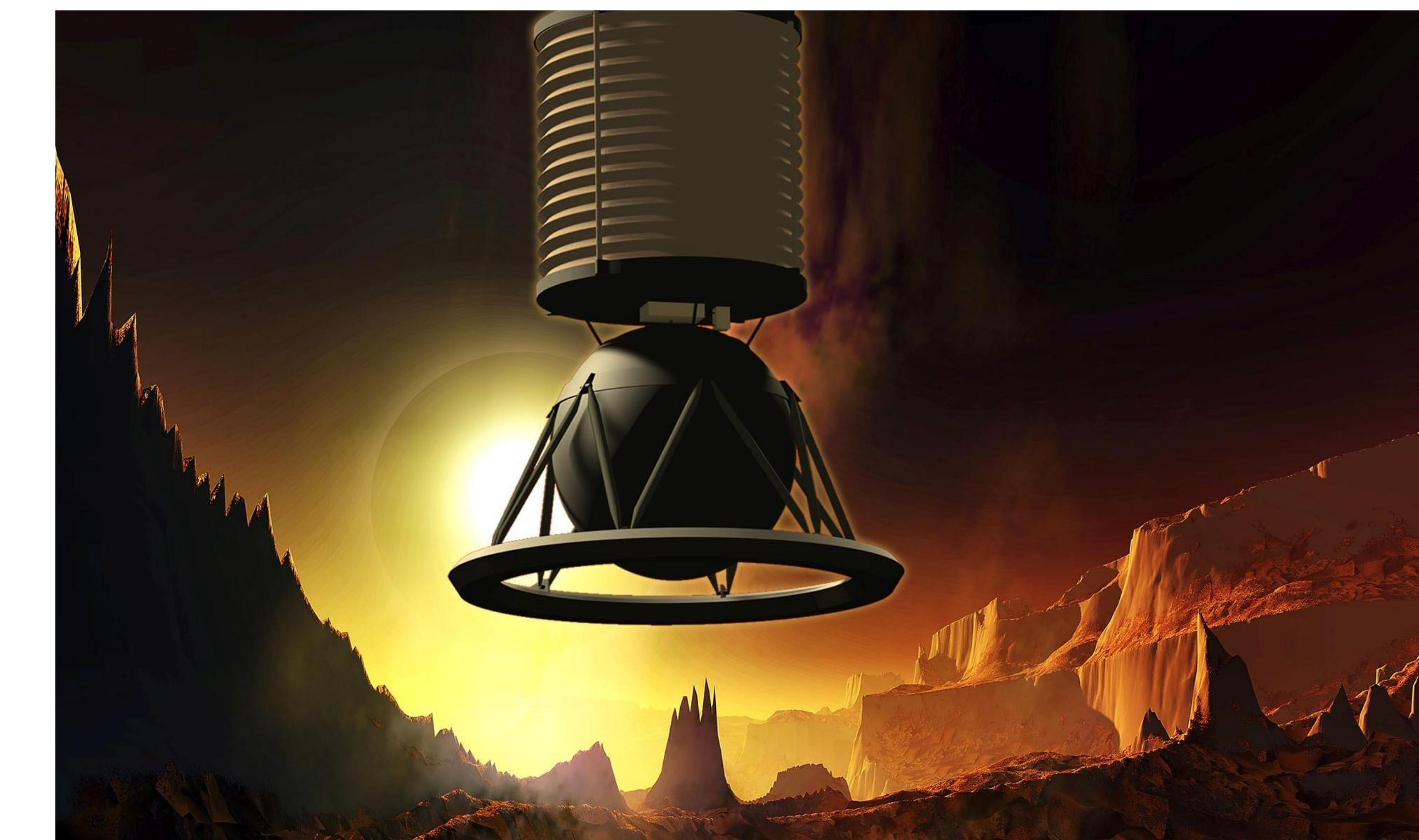
**Additional Flagship Concept:** The evaporated ammonia would also dissociate to hydrogen to supply buoyancy and power from a solid oxide fuel cell operating at ~ 800 C. Oxygen would be carried along to supply the fuel cell. The water produced by the solid oxide fuel cell could be used for additional cooling. This would provide Thermal Control, Power, & Mobility in one package.
