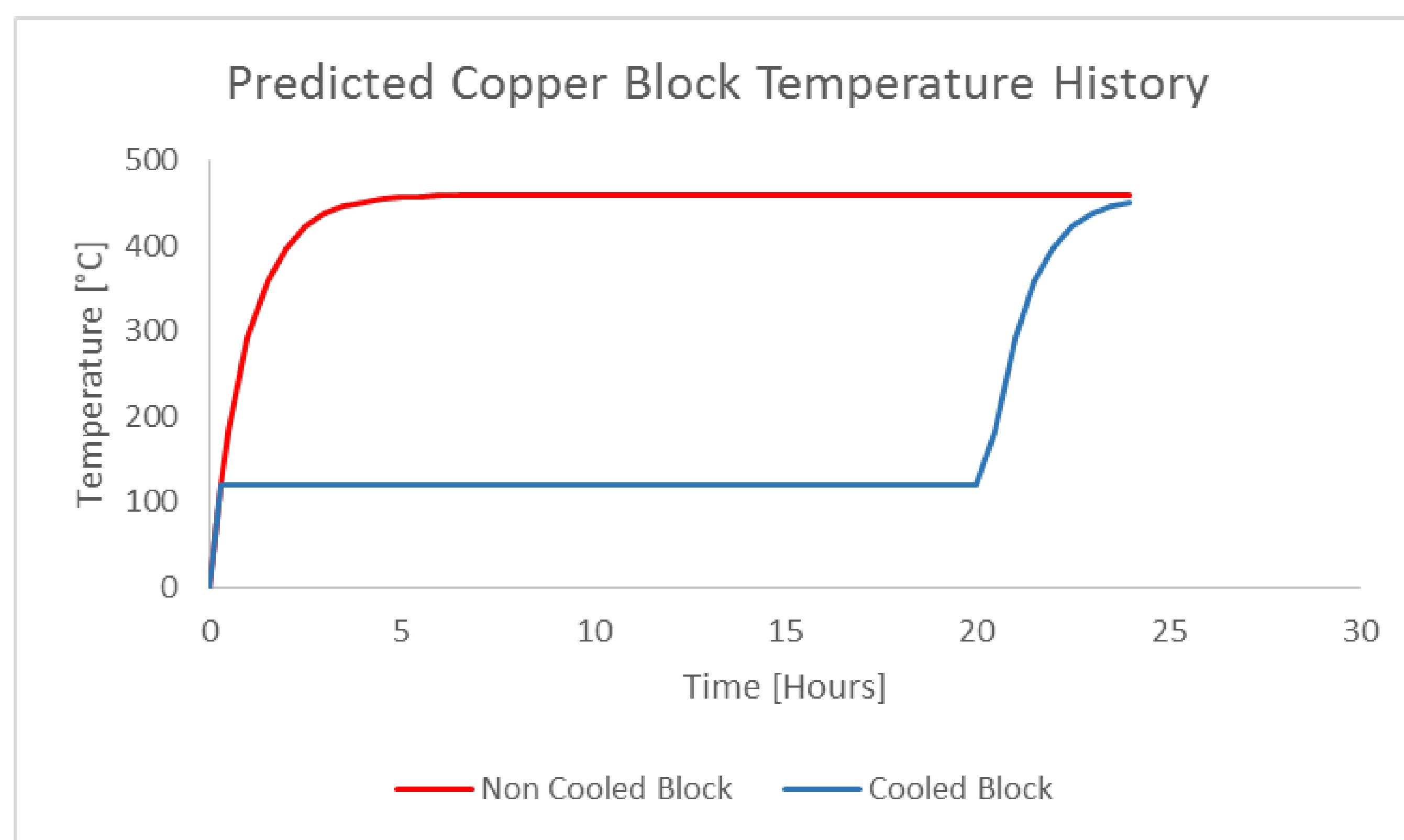
**The Boiling Process.** Boiling ammonia ( $\text{NH}_3$ ) at high pressure is well understood. Testing in the Glenn Extreme Environments Chamber (GEER) (below) would verify the results of the thermal model shown above. Two copper blocks, one cooled by evaporating ammonia and the other without cooling (as a control) would be exposed to Venus surface pressure and temperature inside the GEER.
