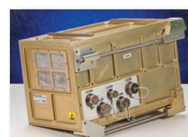
The LMM control box contains the control avionics for the entire LMM subrack facility.
