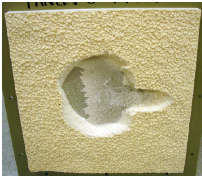
Figure 15.—Damaged foam and exposed Al for test FF100.
