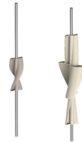
Figure 11: Two potential turbines. The larger one provides significantly more surface area, but comes closer to the cables.
