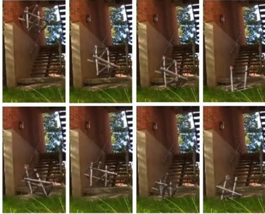
Figure 8: Prototype drop test from 10m – about 14 m/s, greater than its terminal velocity on Titan
