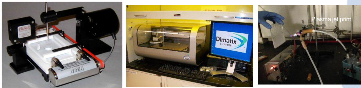
Figure 1 Thin film catalyst deposition apparatus. Left to right: Langmuir Blodgett, nanojet printer, plasma jet printer
