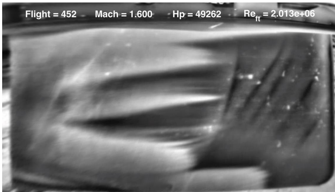
Figure 21. Mach = 1.6 during acceleration at 49,500 ft.
