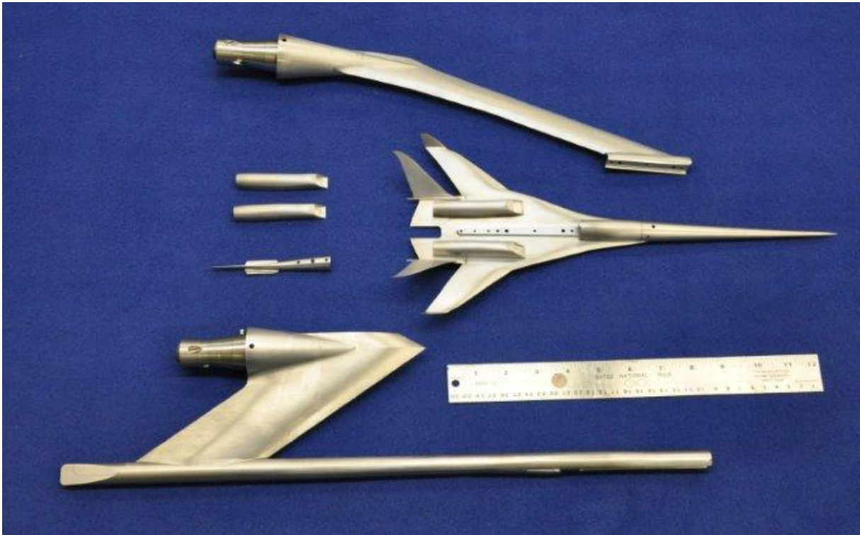
Figure 6-6. Boom parts for the BM model.
