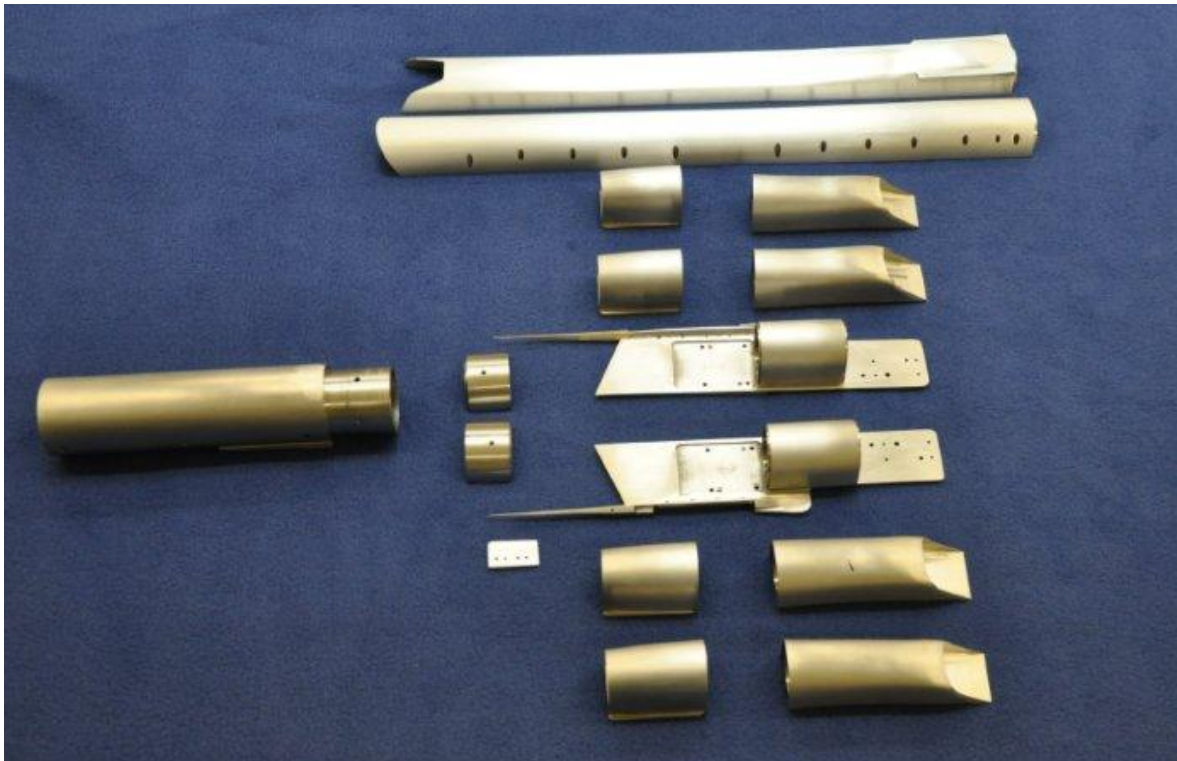
Figure 6-4. Boom and force parts for the PM model.
