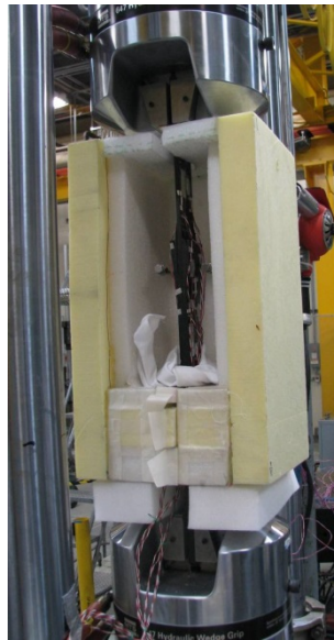
Figure 4. Test specimen encased in thermal insulation box.
