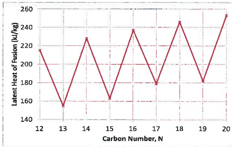
Figure 4. Latent Heat of Fusion of Paraffin ( $\text{C}_N\text{H}_{2N+2}$ ).
