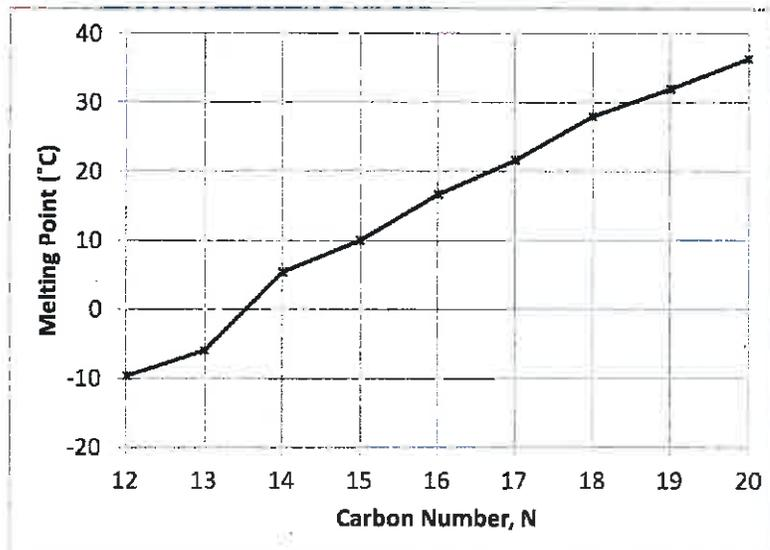
Figure 5. Melting Point of Paraffin ( $\text{C}_N\text{H}_{2N+2}$ ).
