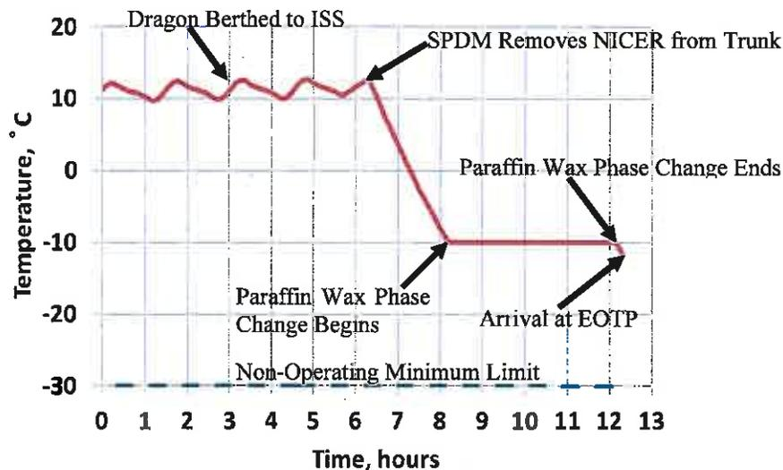
**Figure 11. NICER Temperature Predictions during Removal from Dragon Trunk and Transfer to EOIP.**
