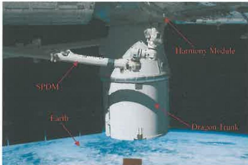
Figure 2. SpaceX Dragon Berthed to Harmony Module on ISS<sup>1</sup>.
