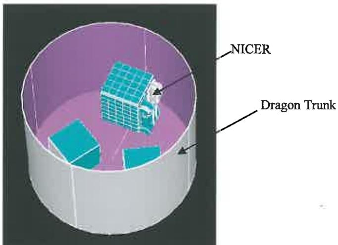
Figure 9. NICER Payload in Dragon Trunk.
