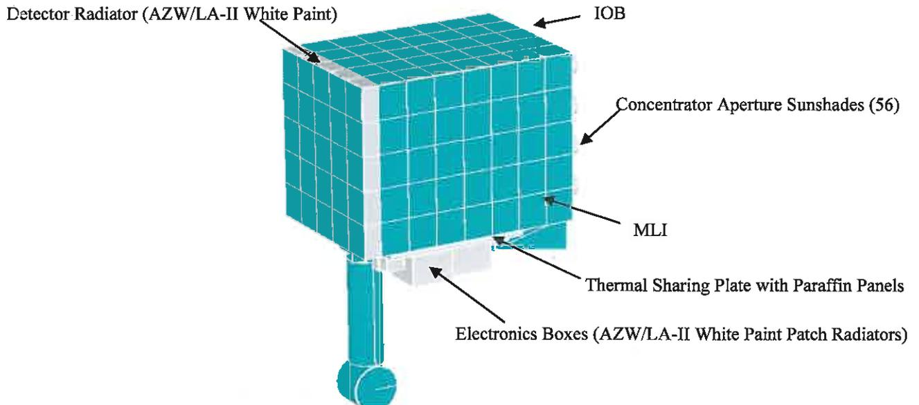
Figure 8. NICER in Deployed Configuration.
