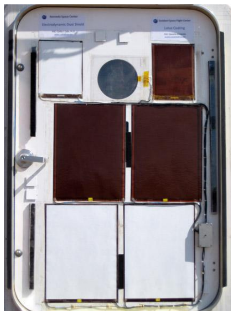
(a) One of the PEM doors with the EDS systems installed
