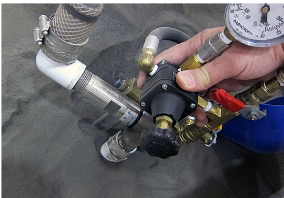
Hand-held Pneumatic Regolith Rake to excavate fluidized regolith. System can also be housed inside a can to contain any dust.
