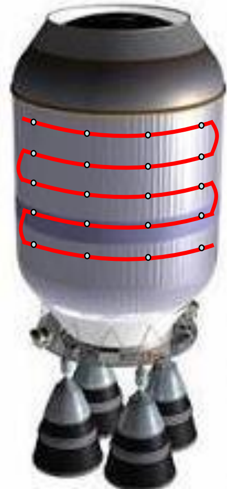
Example hyFOSS fiber layout
