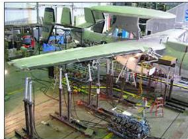
Conventional Loads Calibration Setup
