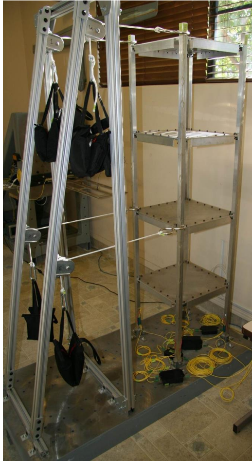
Moment Frame Test Article with FOSS
