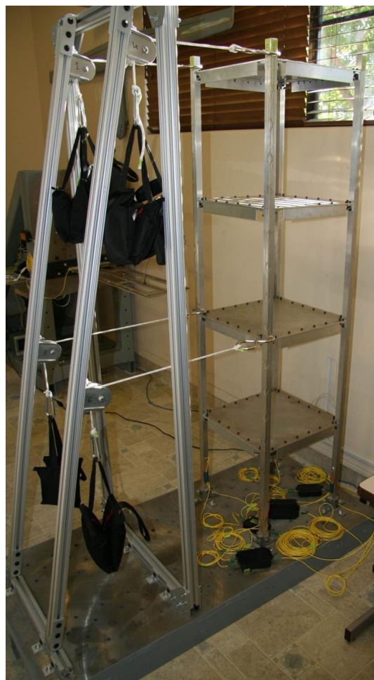
Moment Frame Test Article with FOSS
