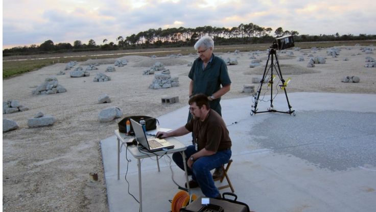
Figure 6. Setup used to laser scan the concrete landing pad following a Morpheus free flight. The laser scanner obtains a topographical mapping of a surface.
