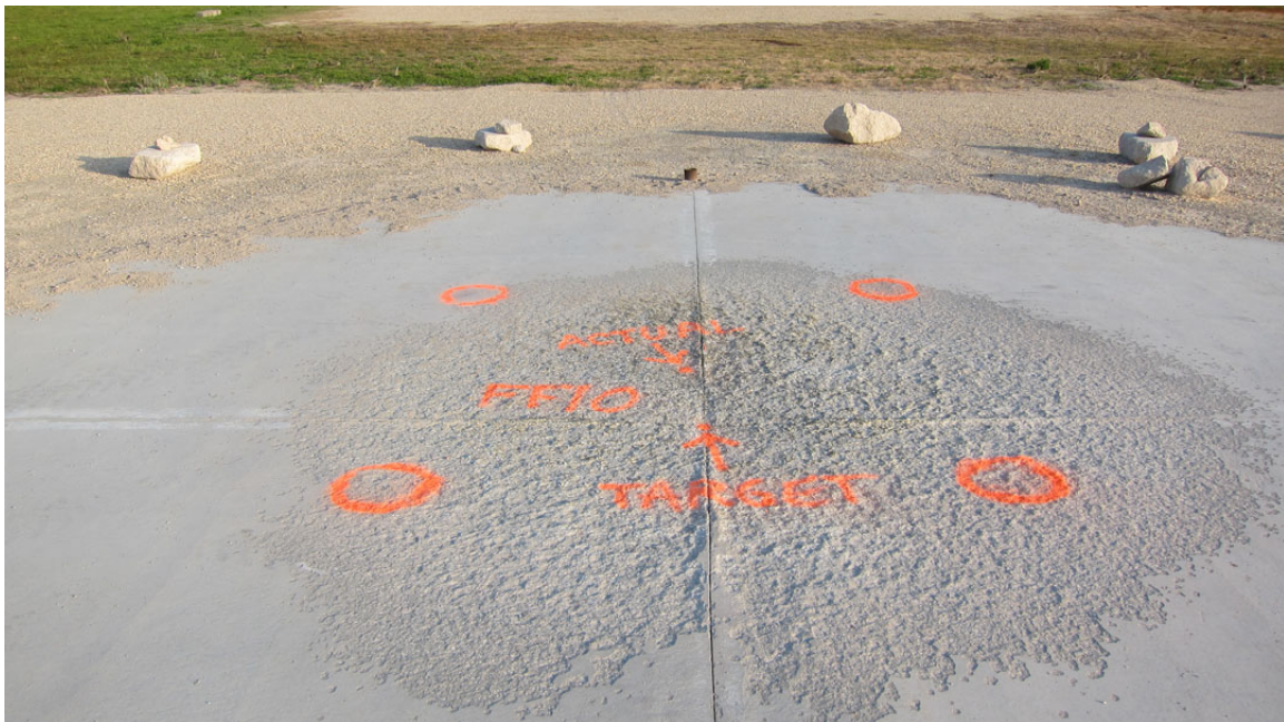
Figure 5. Physical state of the Morpheus concrete landing pad after free flight #10.
