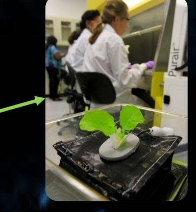
Flight testing of top leafy candidate in Veggie as VEG-03 validation test to fly on Sx-8
