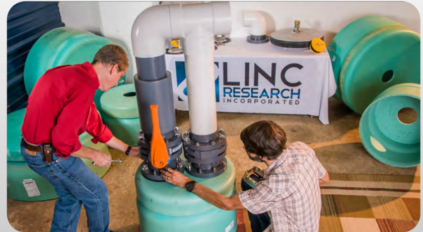
MSFC Inventor Jeff Lindner (left) assembles a fluid damper device for installation in the B2 Building in Brooklyn, NY
