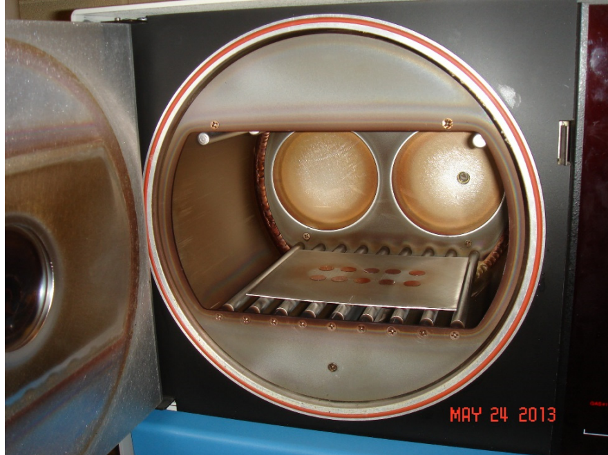
Figure 2.—Samples on a flat plate for directed hyperthermal atomic oxygen exposure in a 35 kHz hyperthermal asher.
