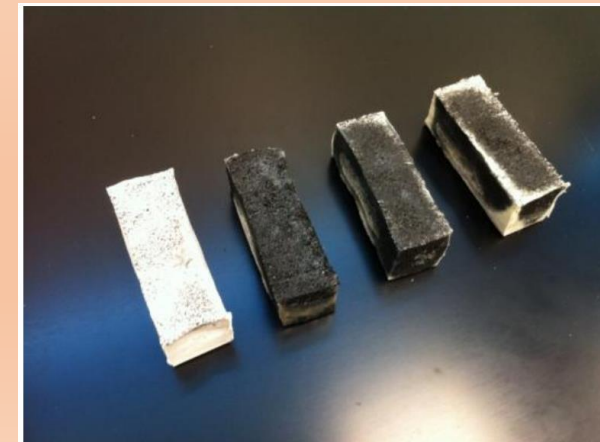
Figure 14. Polyethylene-bound regolith simulant bricks. (Abney et al, 2014)
