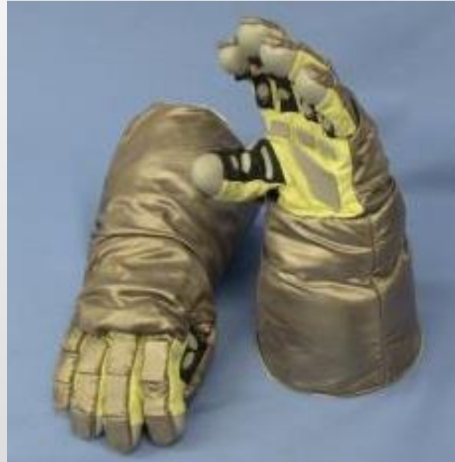
Prototype EVA Gloves with Flexible Aerogel
