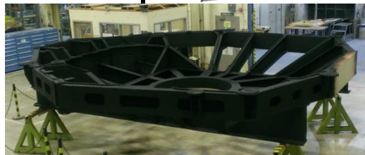
HOSS – Hardpoint Offloader Support Structure In integration in Clean Room
