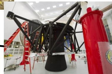
USF Structural Frame – supports Metrology Installed in Chamber
