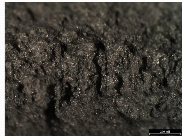
Very rough ductile surface on the surface of the plug fracture area of sample that failed through the plug.
