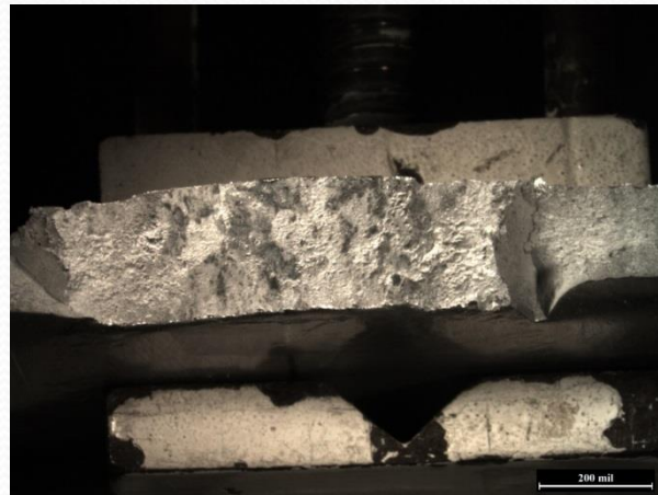
Microscopy of bonded surface of weld and FPW
