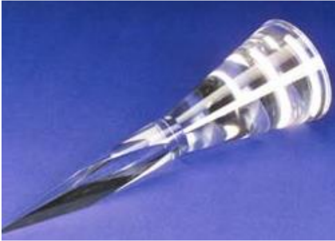
Prototype refractive secondary concentrator made of single-crystal sapphire
