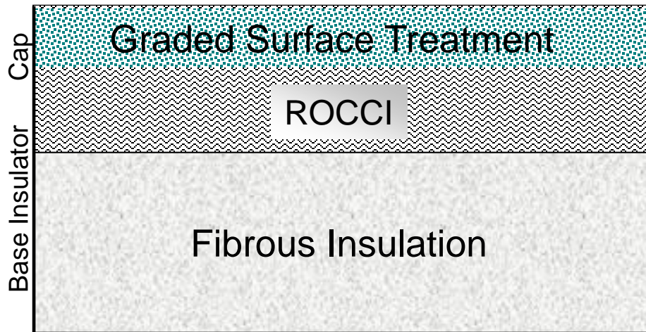
Schematic of TUFROC TPS
