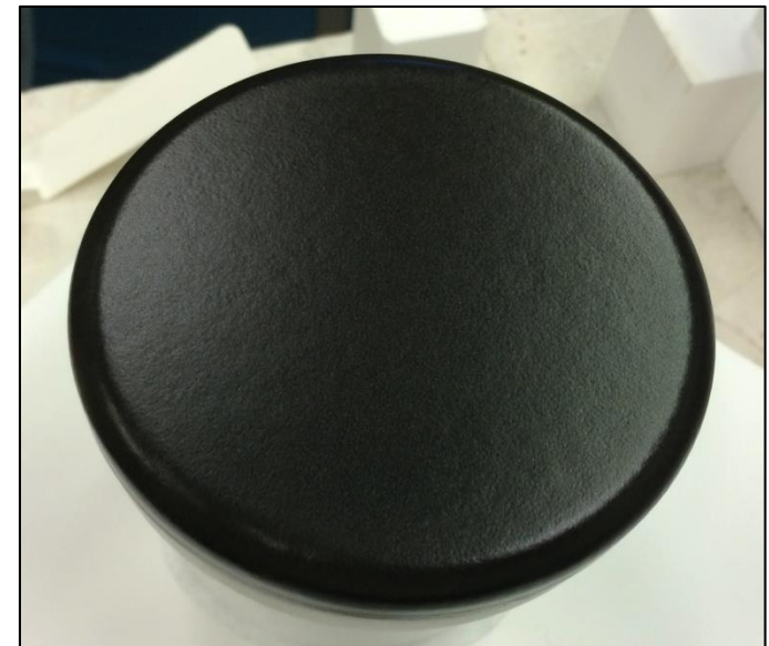
RCG coated tile from an R&D activity
