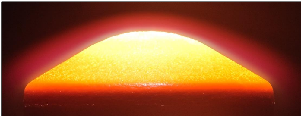
RCG coated TUFROC tile at ~ 3000° F during an arc jet test
