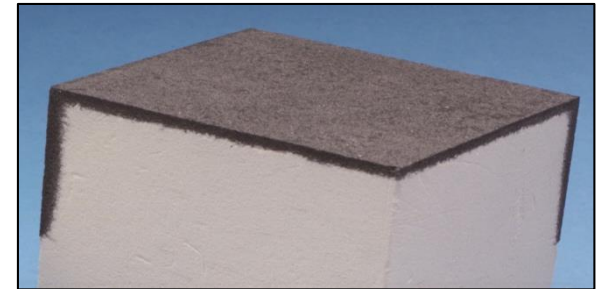
Shuttle era TUF1 treated tile
