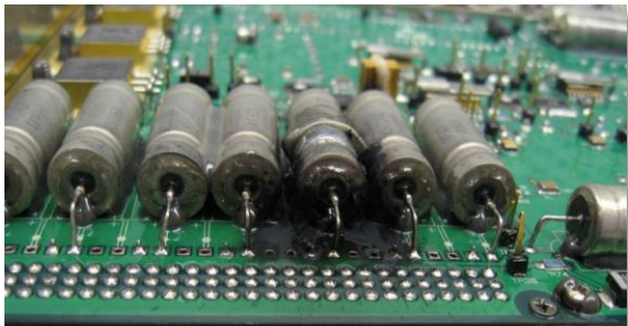
Electrolyte leak due to case rupture resulting in open circuit
