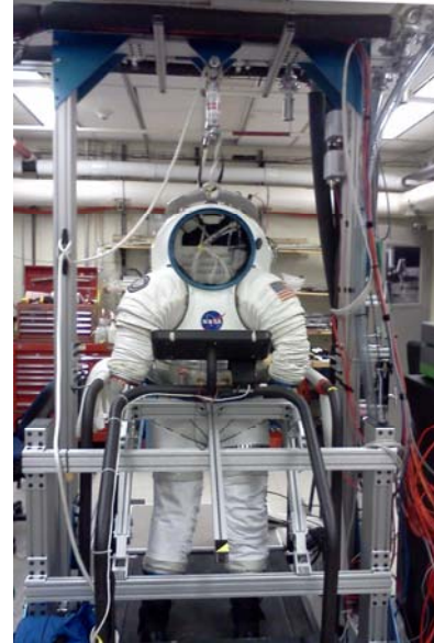
Figure 6. Mark III Suit in Fall Arrest Stand with Don/Doff Fixture
