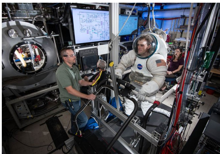
Figure 8. Photo of PLSS 2.0/HITL Testing
