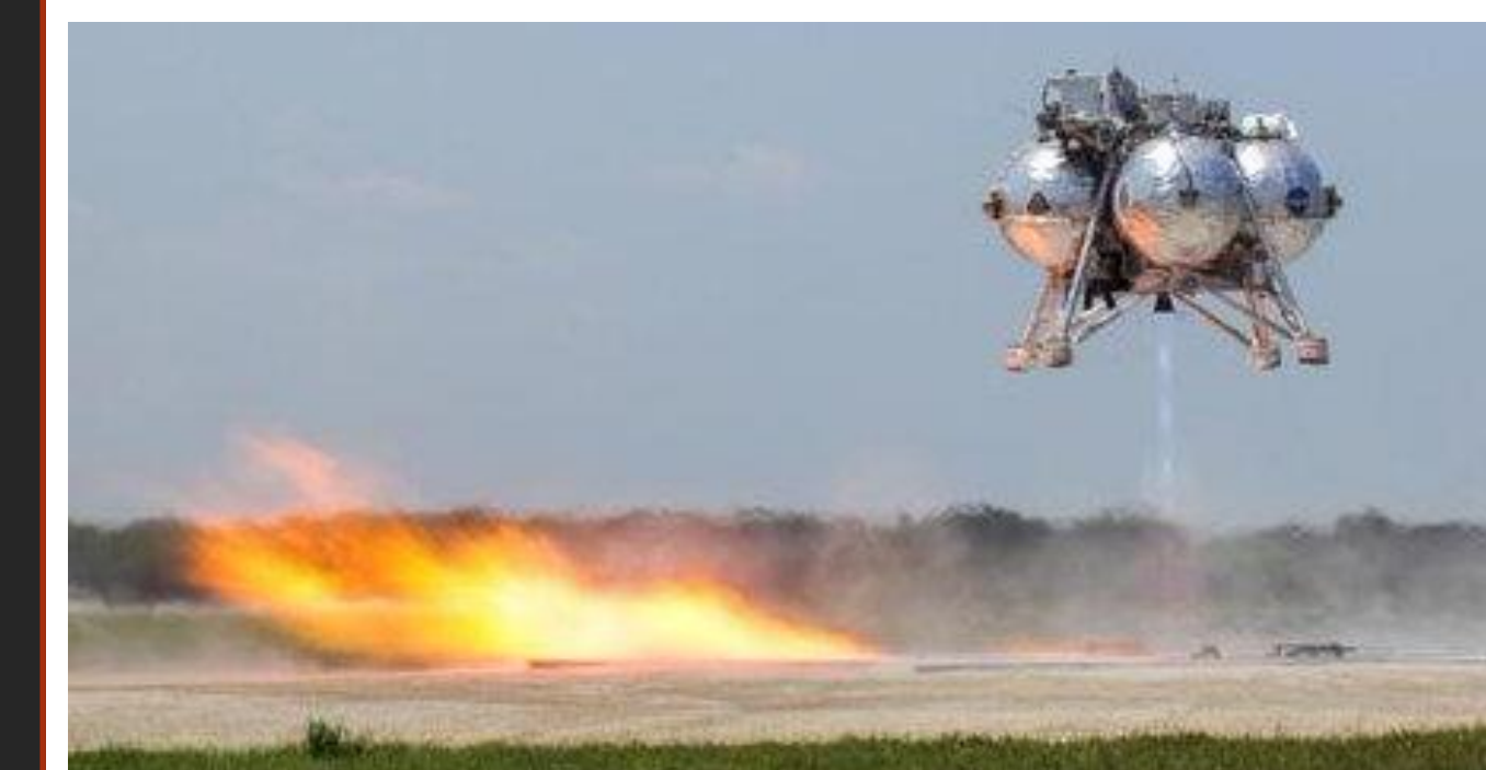
Figure 9: The Morpheus Lander, although not related to Mars Pathfinder, uses a LOX/methane engine.
