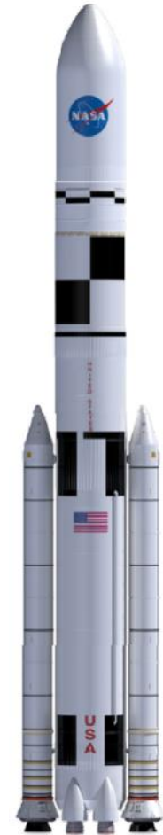
Figure 6. SLS Block 1B with EUS and 8.4m PLF. (Image credit: The Boeing Company)
