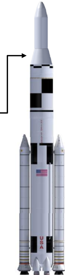
Figure 17. SLS Block 1B with EUS and 5.0m PLF (adapted). (Image credit: The Boeing Company)
