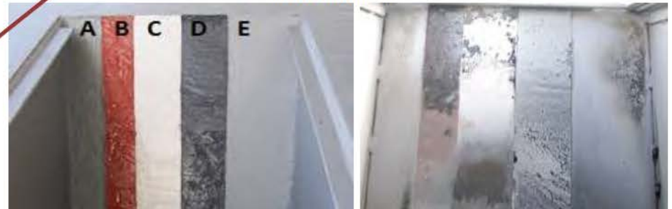
Ablative coatings inside the steel flame trench.
