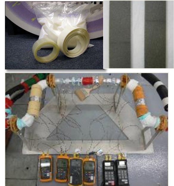
AeroPlastic demo testing on cryo-piping system
