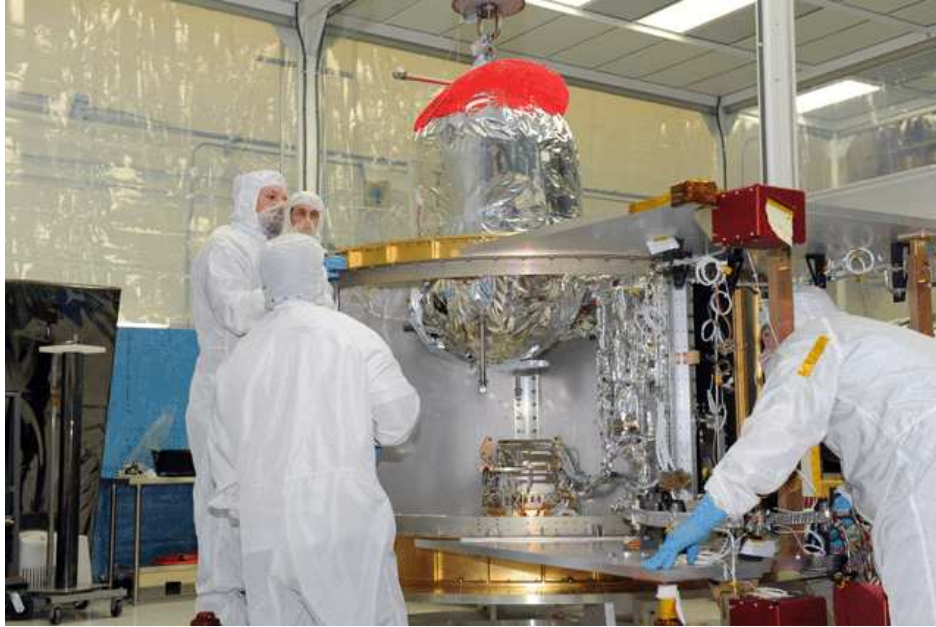
Figure 4.8: The propellant tanks were installed by lowering the tank into the propulsion system structure using a crane. A load cell (not pictured) was placed above the propellant tank to determine the mass of the tank. (Image from [31])
