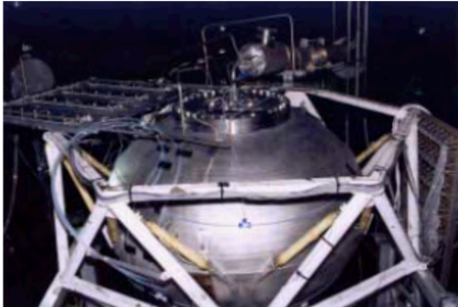
Figure 6. Test article before MLI installation.
