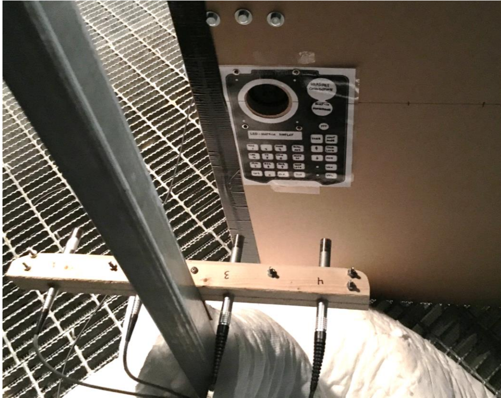
Figure 3: Testing Setup to analyze the Acoustic Diverter
