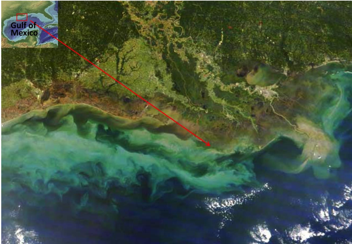
Figure 2.1.1 – The MODIS Spectroradiometer on NASA’s Terra satellite captured this image with a spatial resolution of 250 m 13 days after Hurricane Ike came ashore. The brown areas in the image are the result of a massive storm surge that Ike pushed far inland over Texas and Louisiana, causing a major marsh dieback. Credits: NASA/GSFC.
