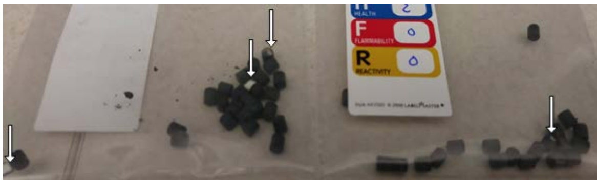
Figure 7. The catalyst pellets that were constricted in packed tubes show signs of physical damage after ten heat shock cycles. The arrows show the damaged pellets from the 450°C heat shock tube (left) and the 600°C heat shock tube (right).
