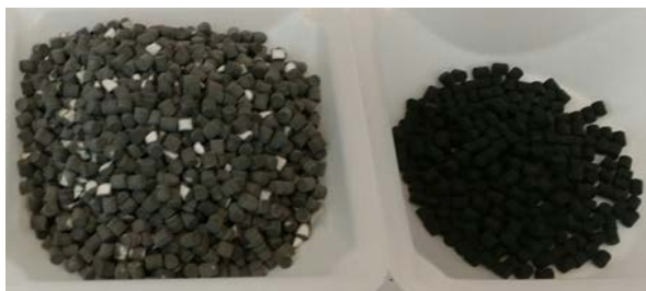
Figure 1. The spent catalyst (left) was removed from the Sabatier reactor after it no longer performed as expected. It is much lighter in appearance and has many broken pellets compared to unused catalyst (right).
