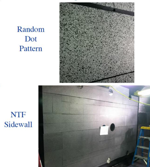
Fig. 1: Randomized dot pattern (top) applied to starboard wall (bottom) of National Transonic Facility for capsule wake RBOS test.
