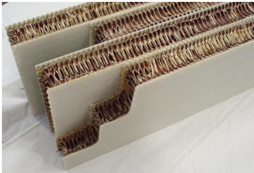
Figure 5. Honeycomb composite panels utilized in design.
