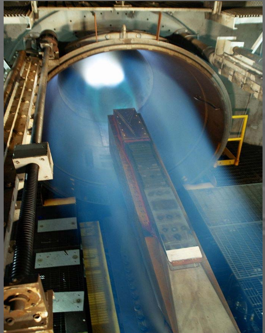
X-51 Engine Test in 8Ft High Temp Tunnel Testing can reach 1927° C
