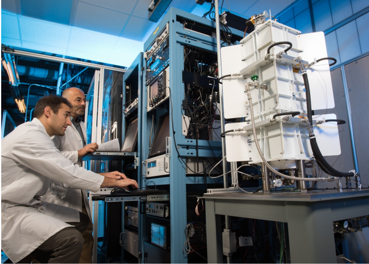
Figure 2.—Advanced Stirling Radioisotope Generator (ASRG) Engineering Unit 2 under test in NASA Glenn Research Center Stirling Research Laboratory.
