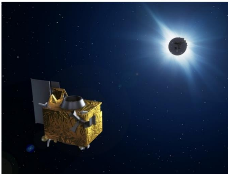
Figure 7. PROBA-3 Spacecraft Aligned to Block Sun Surface Light.
